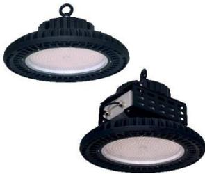
Utilizing custom optic lensing, the CHB is available in three beam distributions: 45°, 90° and 120°. The luminaire comes standard with 120’ of flexible cable and eye bolt for hook mounting. Other mounting options include twist lock receptacles for easy retrofit opportunities or a U-Bracket for conduit, ceiling or wall mounting. Motion sensor, dimming capabilities and battery back-up options are also available.
